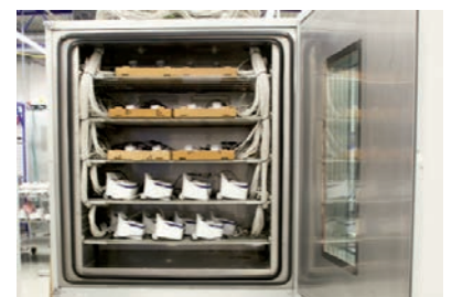
Each camera is tested at extreme temperatures before shipping.
